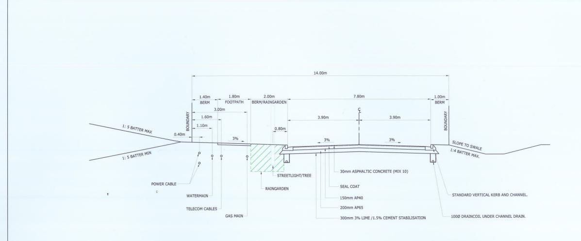
7 TYPICAL CROSS SECTION (PARK EDGE ROAD) AB301 SCALE 1:50 -A1 1:100 -A3 ROAD 4 (CH 85 - CH 200.6)
